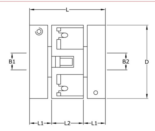
$\begin{array}{lll} B1 & = 8 \\ B2 & = 10 \\ D & = 27 \\ L & = 25.4 \\ L1 & = 9.3 \\ L2 & = 6.9 \\ Screw = M3 \end{array}$
